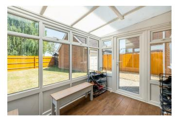
PVC double glazed construction with polycarbonate roof.
